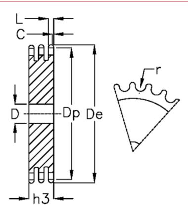
C = 6 D = 40 De = 361.3 Dp = 340.82 For chain size = 2 x 1 1/4 For chain type = 32 B-3 h3 = 146
